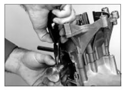
The opening of the snap ring will be positioned at the top or at the bottom, but under no circumstances to the side.
